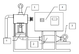
Figure 1. Microwave drying combined with hot air; (1) drying chamber and microwave; (2) the heater; (3) blower; (4) PID controller; (5) electronic balance
